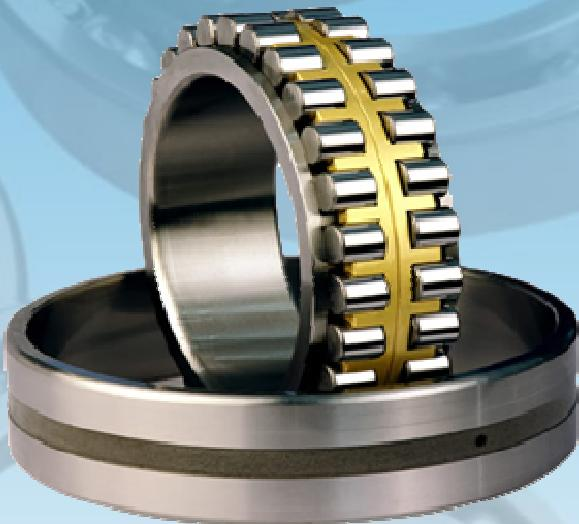
**Cylindrical roller bearings** have rollers that provide a modified line contact with the cylindrical inner and outer ring raceways, while the rollers are guided by ground ribs on either the inner or outer ring. The cylindrical shape allows the inner ring to have axial movement relative to the outer ring. This is especially important when accommodating thermal expansion, where both rings must be press-fitted.
