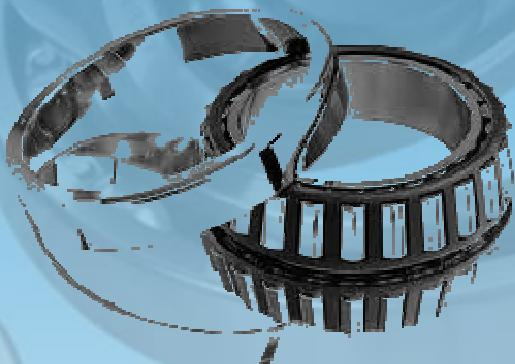
**Tapered roller bearings** utilize conical rollers and raceways, arranged so that the rollers and raceways meet at a common apex. The rollers are guided by contact between the large end of the roller and a rib on the inner ring. This provides high capacity for radial and single thrust loads.
